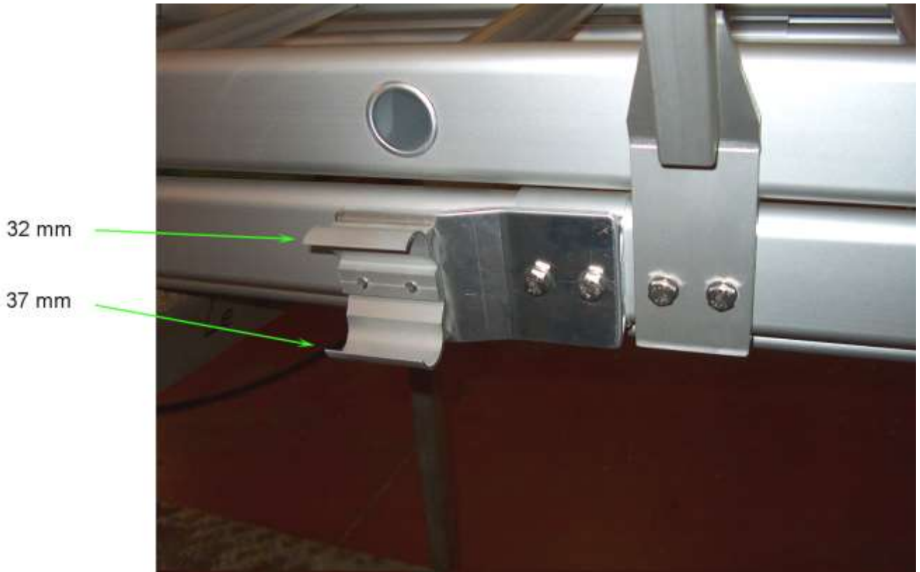
Fig. 5. Counterweight sheath bracket mounting.
